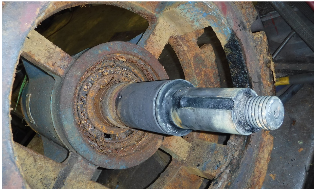
Image 2- Rusted Radial Bearing
